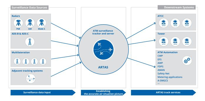
Figure 2: Schematic of ARTAS inputs and outputs
